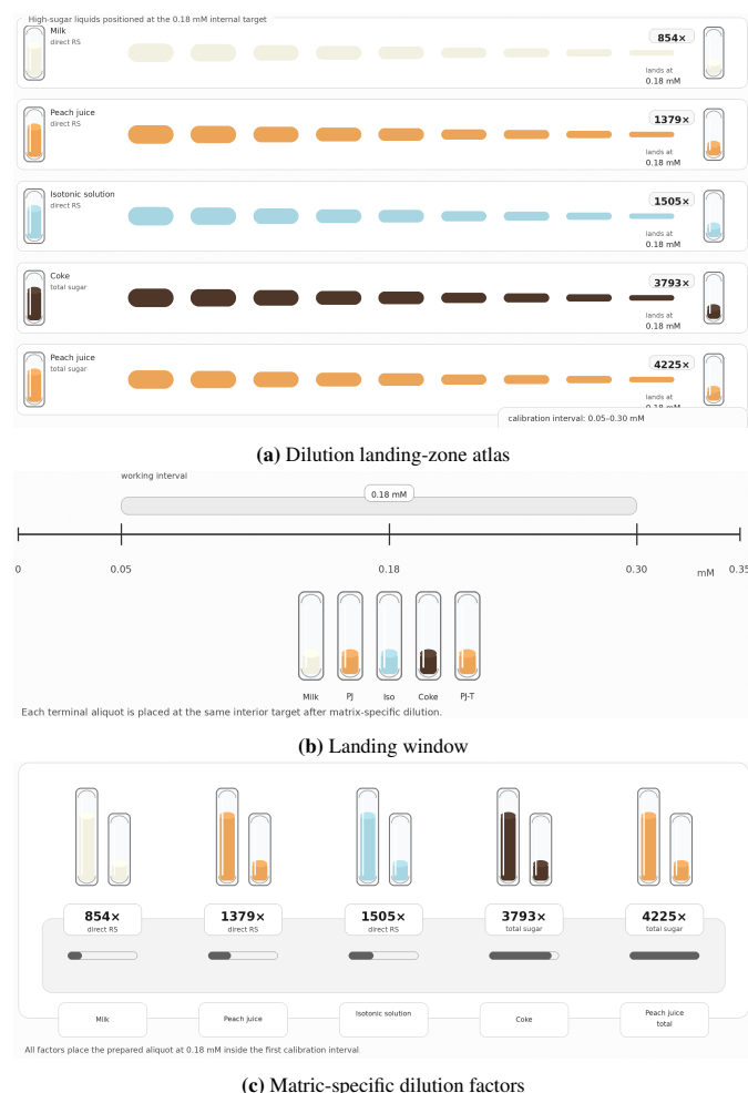
Figure 7: Dilution placement for liquid food samples.
